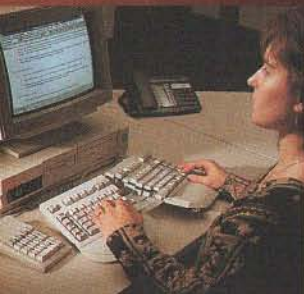
Keyboard split at an angle of 30° with steep roof inclination and optional numeric pad on the left.
